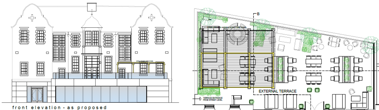
Images 2 & 3 Proposed Elevation and Plan showing scaled back canopy proposal occupying smaller section of terrace
